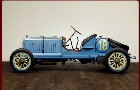
1908 Panhard & Levassor Q-Type Race Car 50 hp T-40 engine, chain drive
